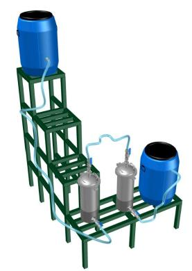
The unit consists of a filtration vessel and an activated carbon vessel. For water production the unit just needs to be connected to a higher located raw water tank. The raw water will enter the unit by gravity and will be cleaned by the ultrafiltration membrane cartridge and the activated carbon. Water production is up to 8,000 L/day per unit.
