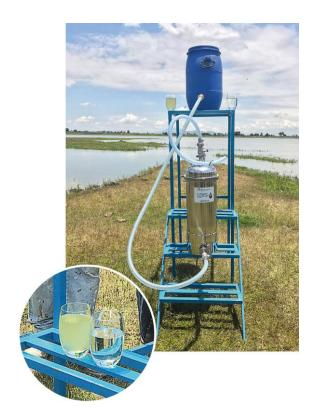
The skid consists of a filtration vessel with integrated ultrafiltration membranes. For water production the skid just needs to be connected to a higher located raw water tank. The raw water will enter the skid by gravity and will be cleaned by the ultrafiltration membrane cartridge inside the filtration vessel. Water production is up to 8,000 L/day per unit.
